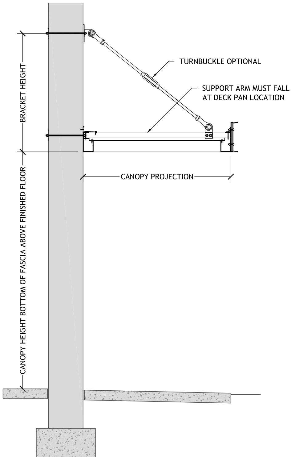
**CLEVIS ARM OVERHEAD SUPPORT 8 INCH FASCIA GUTTER PAN AND CAP DECK
