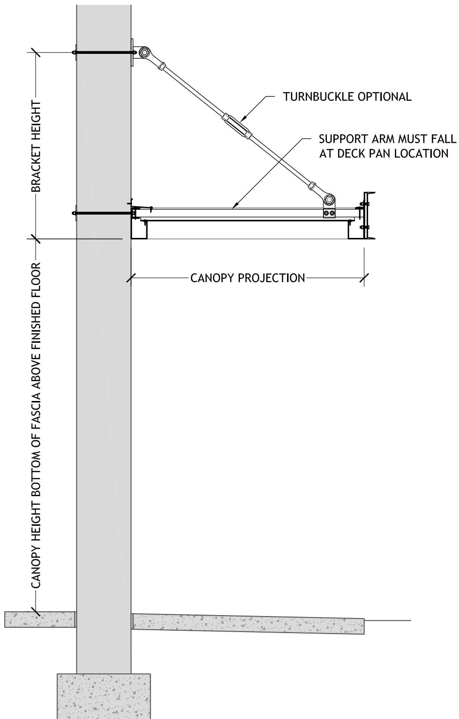
**CLEVIS ARM OVERHEAD SUPPORT 8 INCH FASCIA GUTTER FLUSH DECK
