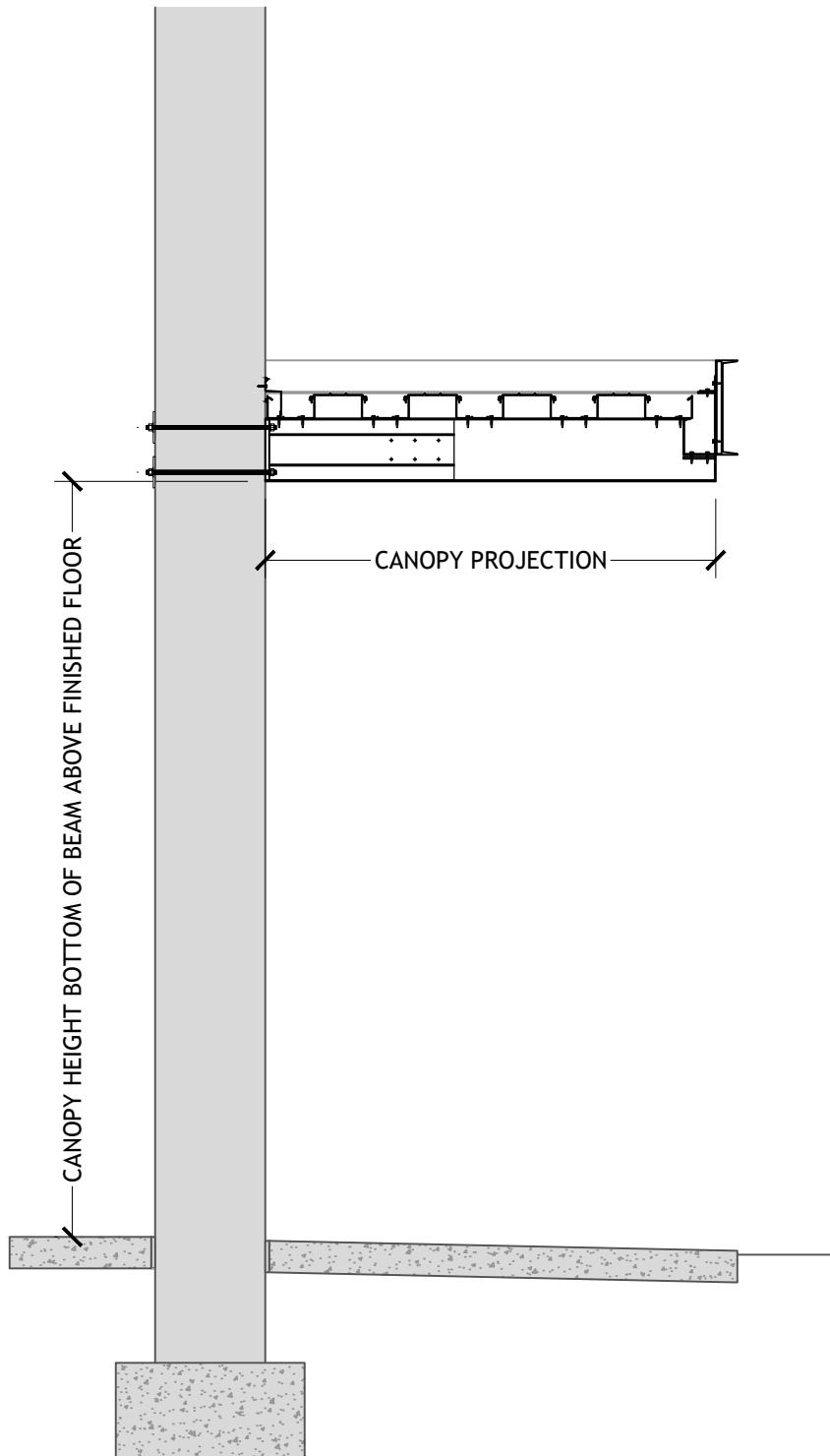
**FACE MOUNT BOOT SUPPORT 8 INCH FASCIA GUTTER PAN AND CAP DECK
