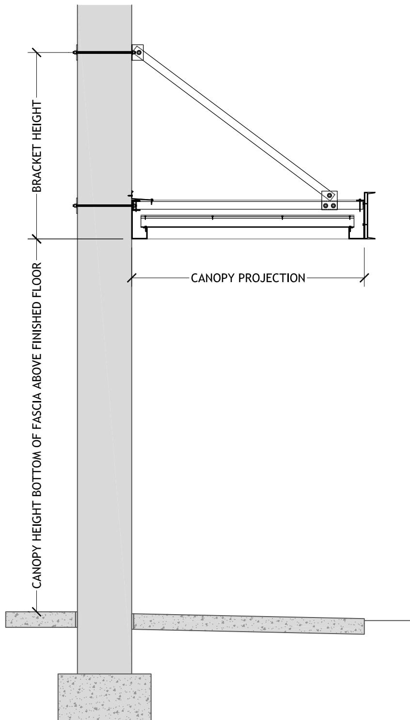
**STANDARD OVERHEAD SUPPORT 10 INCH FASCIA GUTTER PAN AND CAP DECK
